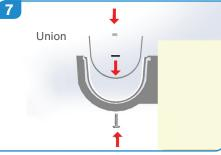
Push bolts through the sole of the gutter from the underside and position union into the gutter ensuring that the slotted holes in the union are filled with sealant as the union is pressed into place. Apply nuts and washers and gently tighten (Do not overtighten as this may force the sealant out of the joint).
