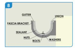
Clean off any excess sealant to either side of the joint or apply additional as required to create a smooth bead.
