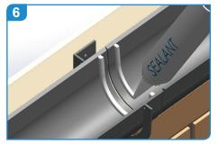
Ensure that all fixing surfaces are clean and dry. Apply 6mm bead of low modulus sealant to each side of the joint.
