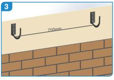
We recommend fixing brackets every 750mm and using an additional bracket for each outlet or angle.
