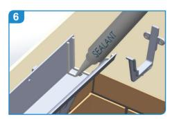
Ensure that all fixing surfaces are clean and dry. Apply 2 x 6mm beads of low modulus sealant into the plain end of the gutter, place the spigot end of the gutter length into sealant.
