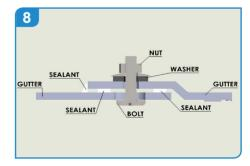
Clean off any excess sealant to either side of the joint. Apply additional sealant as required to the internal face only to create a smooth bead.
