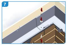
Push bolt through the sole of the plain end of the gutter from the underside and position spigot end of gutter directly over joint. Ensure that the slot is filled with sealant before applying nut and washer, gently tighten. Do not overtighten as this may force the sealant out of the joint.
