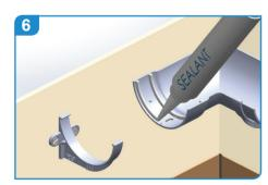
Ensure that all fixing surfaces are clean and dry. Apply 2 x 6mm beads of low modulus sealant into the socket end of gutter, place gutter length into sealant/socket.
