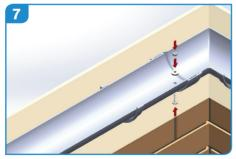
Push bolt through the sole of the gutter socket ensuring that the slot is filled with sealant before applying nut and washer, gently tighten. Do not overtighten as this may force the sealant out of the joint.
