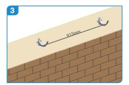
We recommend fixing brackets every 915mm and using an additional bracket for each outlet or angle.
