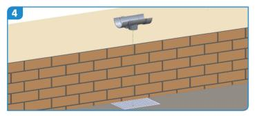
With the use of a plumb or laser line, position outlets over gullies and support with at least one bracket. Also include a bracket per angle (internal or external).
