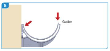
When fitting outlets and angles position the rear face of the gutter underneath the roof finish. Locate the gutter into the fascia bracket and then clip the front edge down into position.
