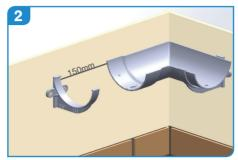
Image 2 shows the ideal bracket positioning for the angle and bracket to take the gutter length. (Max 150 mm from joint).
