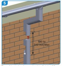
Top of last pipe is required to finish 180 - 340 mm max beneath the offset.
