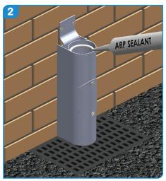
As per local building regulations, if a shoe is not installed access pipes should be fitted and positioned to give suitable rodding access as required.
