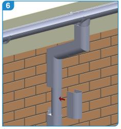
Once connected place cover position over telescopic section using 2 beads of sealant to fix in place.
