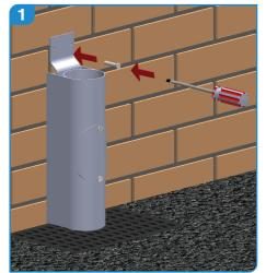
Ensure vertical alignment between drain and gutter outlet. A drain adaptor or offset may be required to terminate the pipe work into the gully. Slide the main fixing plate into the top of the pipe, attach clamp and secure with M6 nuts supplied. Fix to the wall using plastic wall plugs and stainless steel screws (dependant on substrate).
