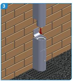
Position next pipe and fix back with 2 No. fixing screws.
